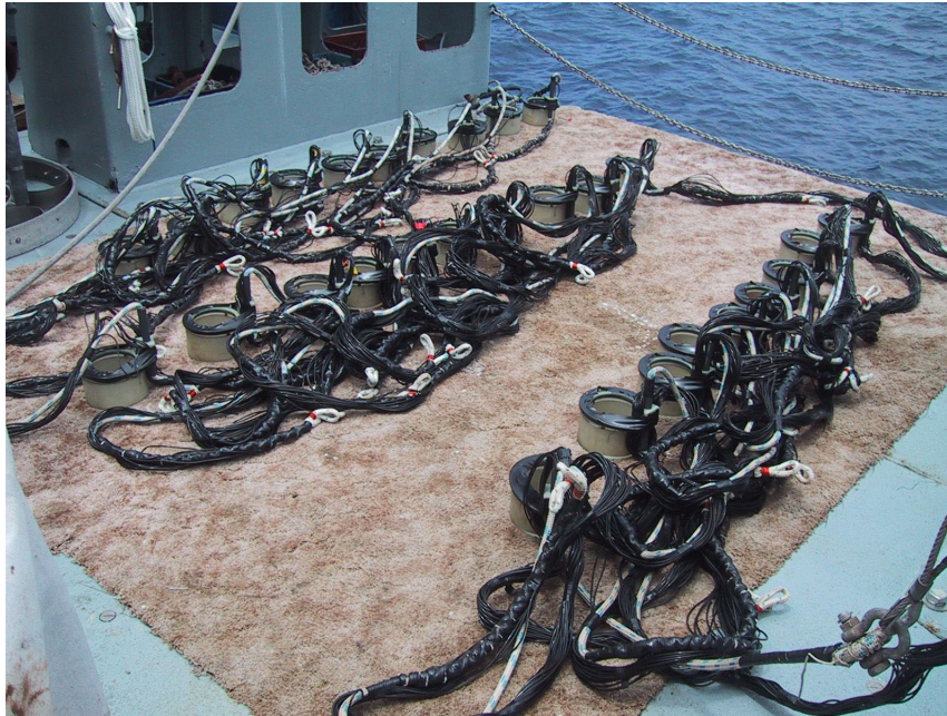
Figure 20. Photograph of 29-element source-receive array.
