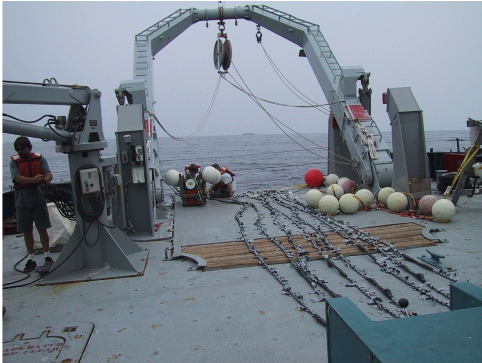
Figure 22. Photograph of 16-element, autonomous receive array.
