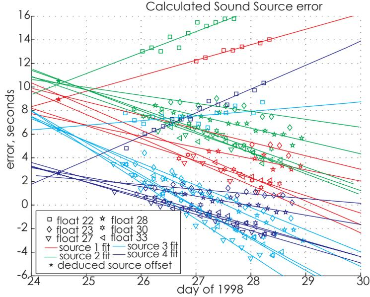
**Figure 10.** Returns for the first windows, coded by color for sound source and symbol for float number. Linear fits for each float/source pair are shown as colored lines. Sound source clock offset shown as solid stars.
