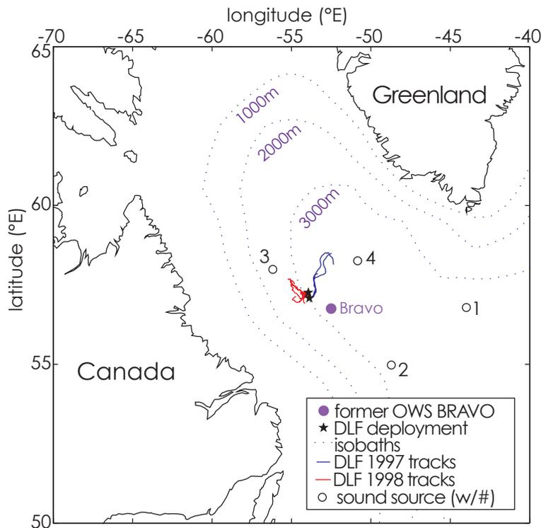
**Figure 9.** The Labrador Sea, with bathymetry shown dashed, the former BRAVO site indicated, the four RAFOS sound source locations shown as numbered circles, the DLF deployment locations shown as stars, and DLF tracks shown as colored lines (red for 1998 and blue for 1997)
