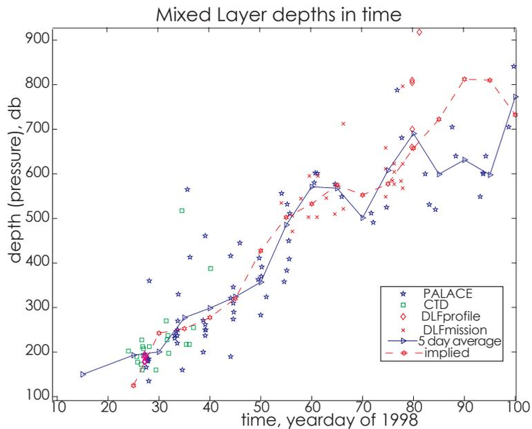
**Figure 7.** Mixed layer depth as in Fig. 5. “x” symbols mark data collected during the Lagrangian portion of DLF mission (within the mixed layer). Diamonds mark DLF (non-Lagrangian) profiles. Dashed line is “implied” depth, i.e., CTD Station 6 pressure at “background” potential density.
