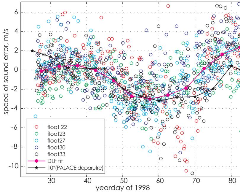
**Figure 11.** Calculated  $c_{err}$  for every window with signals from three RAFOS sources detected. Circles are data color-coded by float. Magenta line is fit of the DLF data with a five-day running mean. Black line is ten times the PALACE float depth-averaged  $c$  variability.
