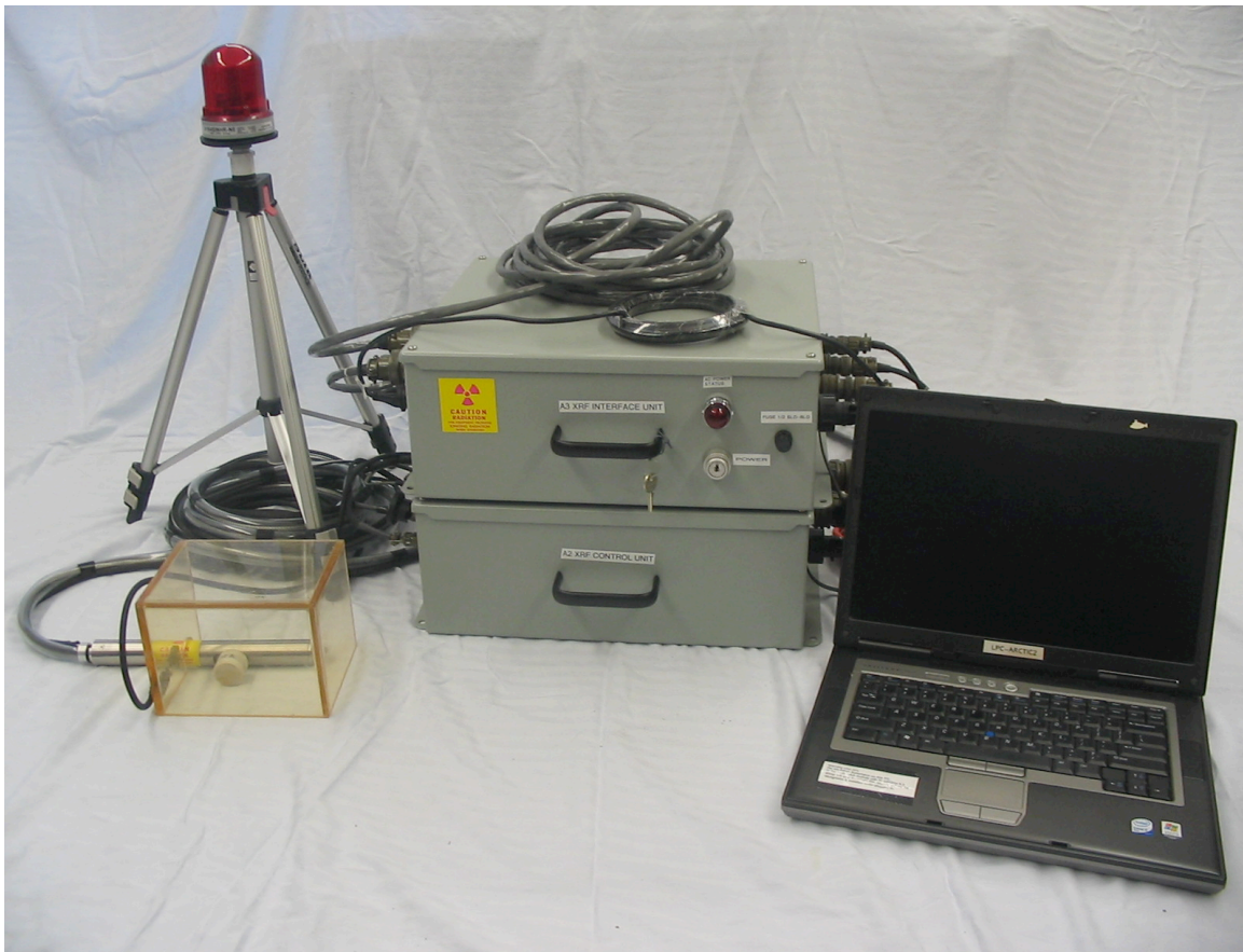
Figure 2. (from left to right) Borehole XRFs Head Unit , X-ray warning light, umbilical cable, X-ray Interface and Control units, and laptop computer.
